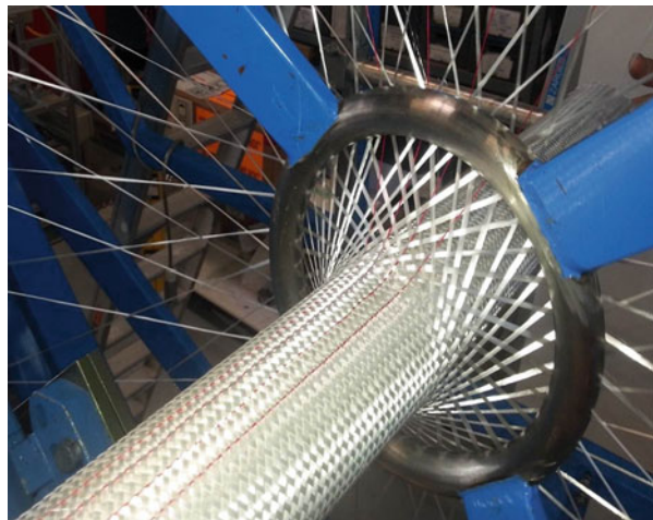
Fig. 6 Glass fiber fabric with integrated FOS as longitudinal fiber (red) (Preisler 2020)
