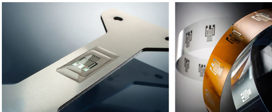
Fig. 7 Encapsulated strain gauge (half bridge) on a metal component (left) and on temperature-sensitive polymer films (right), manufactured using additive printing and laser processes (source: Fraunhofer ILT)
