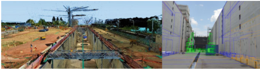
Fig. 3 New Trier lock: left: Colored point cloud of a laser scanner, right: digital as-built model
