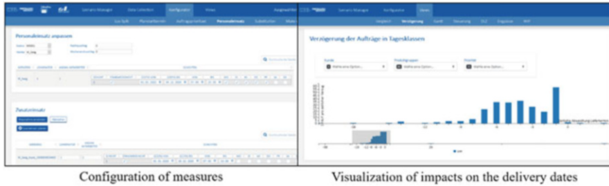
Fig. 6 Simulation-based “EkuPro” tool for the objective selection of countermeasures upon disturbances in production (source: WZL of the RWTH Aachen)
