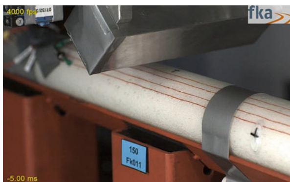
Fig. 8 Inducing damage within a drop tower test (Preisler 2020)
