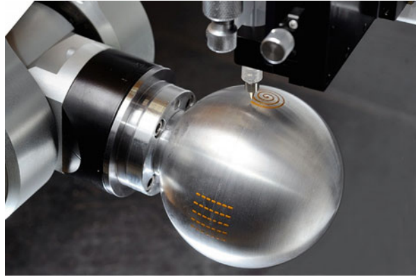
Fig. 9 Additive manufacturing of electrical functional layers on a 3D component using printing and laser processes (source: Fraunhofer ILT)
