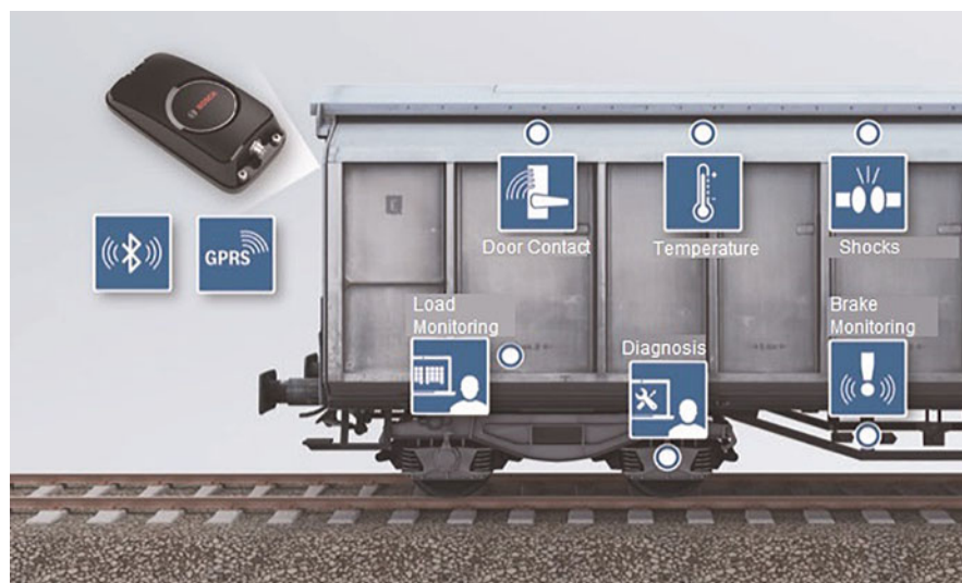
Fig. 16 Digital train monitoring with wireless transmission equipment (© Bosch Engineering GmbH)
