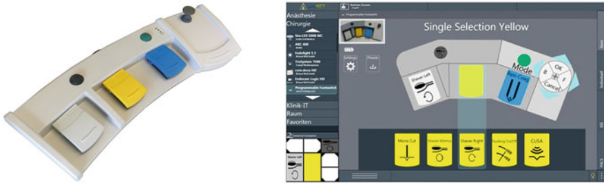
Fig. 5 Universal foot switch (left) and function assignment via the GUI (right)
