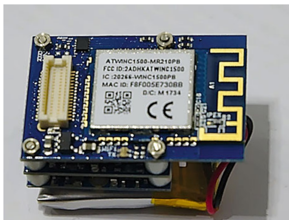
Fig. 3 One example of an inertial sensor used for motion analysis. The sensor consists of a WiFi-shield, a micro-controller, an inertial sensor shield, and a lithium-ion-battery. The sensor weighs about 35 g
